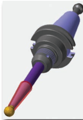
Set clearances for any part of the tool or holder
